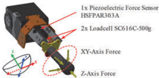
Fig. 2 Placement of sensors and hemisphere sensing range
