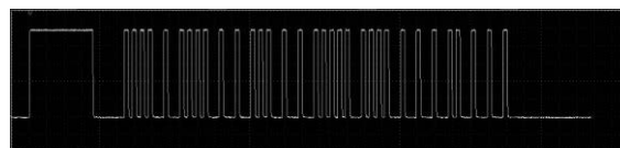
Fig.11 Wave form of button “1” pushing.
