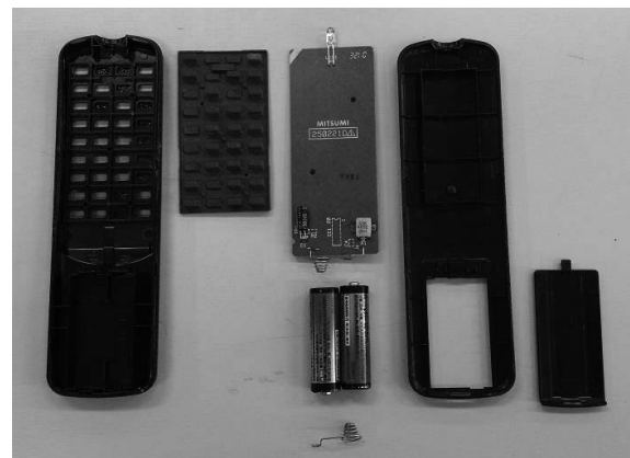
Fig.17 Teardown of an IR TV remote controller.
